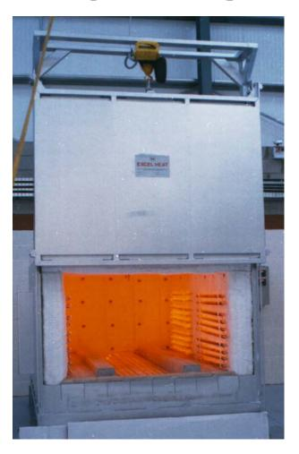
This low thermal mass insulated electrically powered furnaces has a maximum working temperature of 1000 Degrees C (1832 F) with purpose built high temperature hard wearing load bearing piers, which supports the baths once in the furnace.
